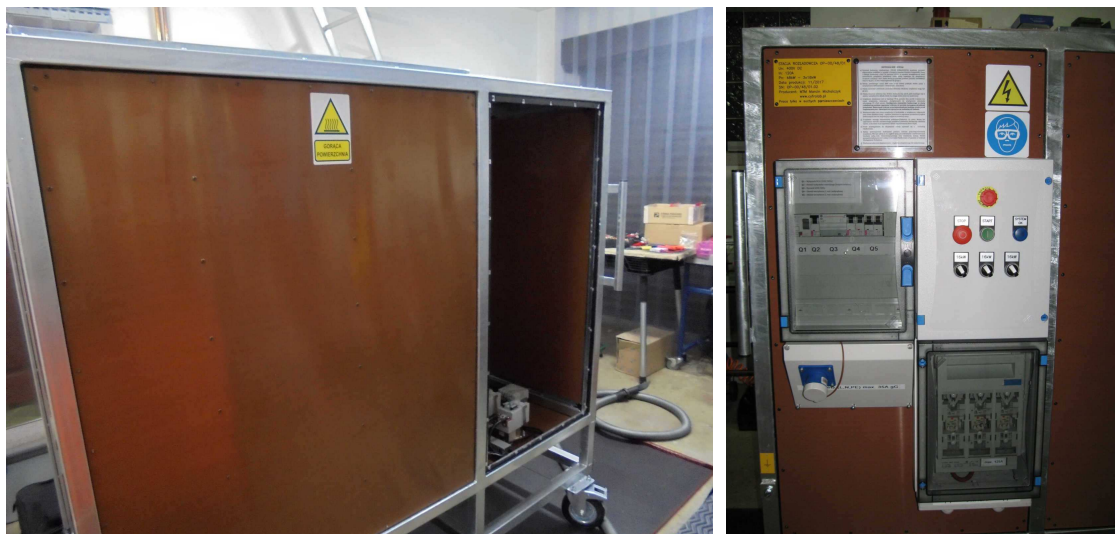
Rys. 1 P_n = 48\text{kW} - 3 \times 16\text{kW} ; U_n = 400\text{V DC} ; I_n = 120\text{A} .
